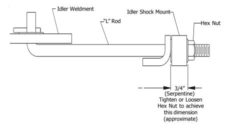
Note: Belt deflection or movement should be approximately 1/4" when measured at mid-point between pulleys. Periodically inspect both belt and idler systems.
